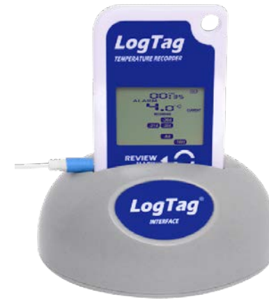
Figure 5: TRED30-7 in standard USB interface cradle LTI/USB
