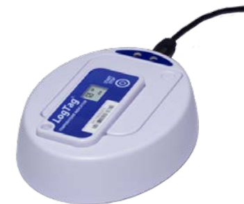
Figure 6: TICT in LTI/USB-TICT interface cradle
